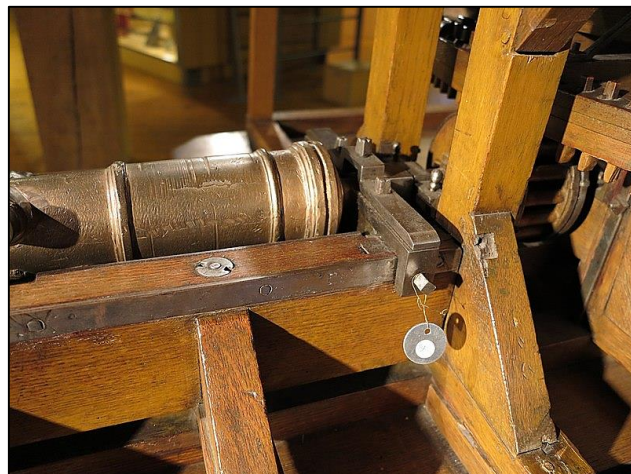
Model of the horizontal boring machine the Verbruggens developed on display at the National Military Museum in Amersfoort, the Netherlands.
